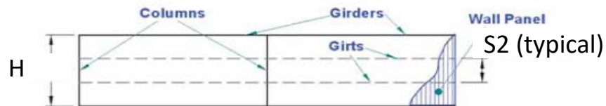
Fig. 2-10. Steel building—elevation view.
