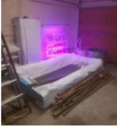
Figure 9 – bamboo passive soak for 1 week
